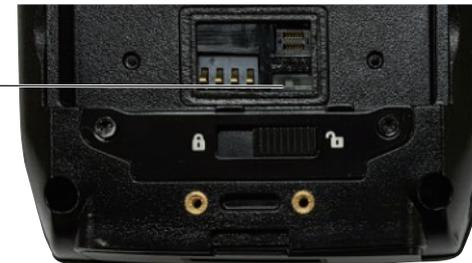
To attaching main battery to the back battery compartment of the PDA.
