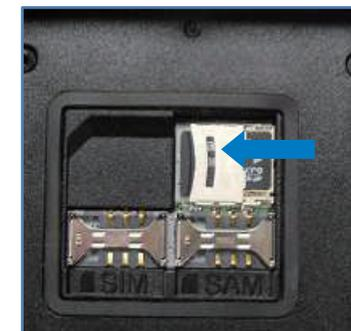
Push the cover up as arrow direction to lock it, and attach the main battery and turn on the power.
